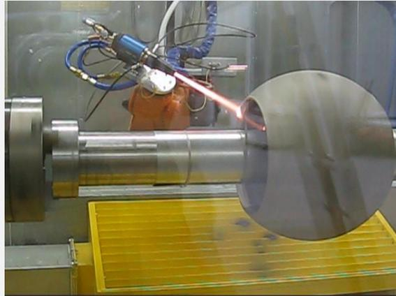
Consists in the melting and acceleration of the spray particles by high pressure combustion of fuel and oxygen and spray through special designed expansion nozzles that lead to supersonic gas and particle velocities (up to 900m/s).
