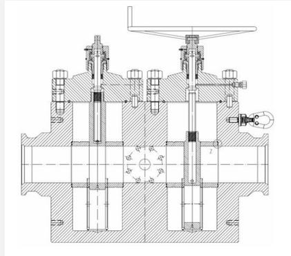
Gate valves are pigable in their full-bore version, which means that a pig can pass the valve without interruption.
