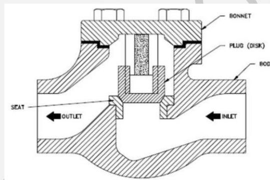
**Piston check** valves are used to avoid problems in the piping and pumping systems (cavitation) avoiding any reversal of the flow. They are opened by the passage of the fluid and use a spring to close them. They also keep the pipes full of fluid if the pumping equipment is stopped.
