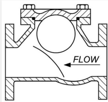
The **lift check valve** has a seat design like a globe valve. The disc is generally in the shape of a piston or a ball.
